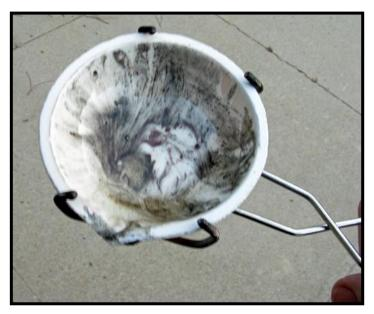
When the dish is hot, sprinkle in a half teaspoon of borax, let it melt, and spread it with a carbon rod over all of the interior surface of the dish. Add more borax if needed.
